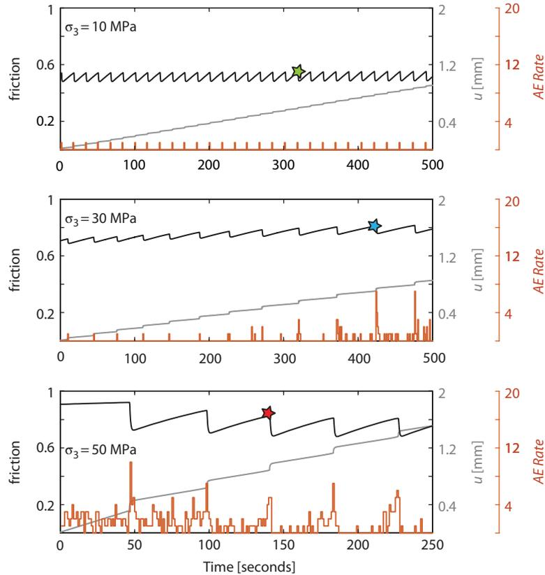
**Figure 12.3** Evolution of resolved friction coefficient, displacement, and acoustic emissions rate during stick-slip sequences conducted at 10, 30, and 50 MPa confining pressure. Black, grey, and red solid lines correspond respectively to the friction coefficient, the axial displacement, and the AE-rate (AE/s). Colored stars refer to individual main shocks presented in Figure 12.4. See *electronic version for color representation*.
