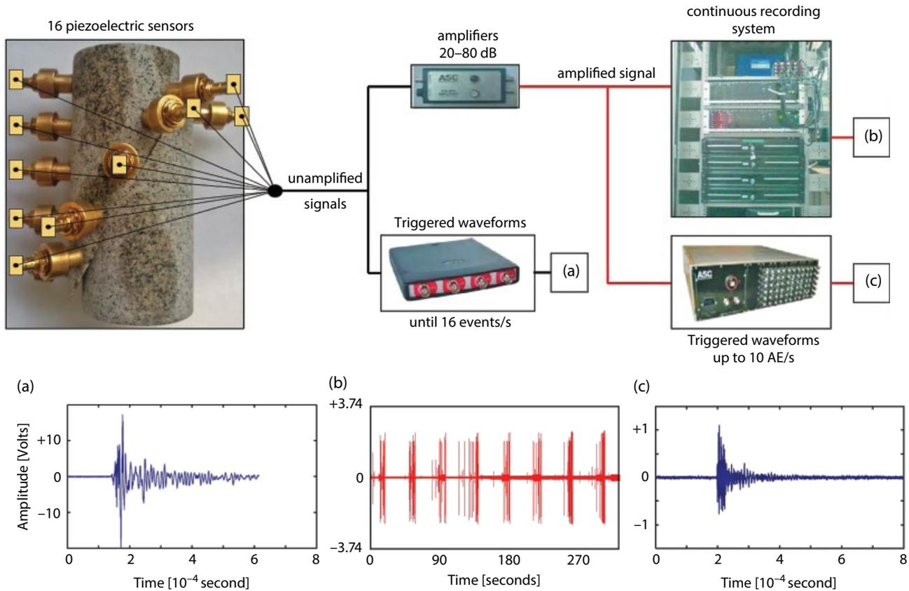
**Figure 12.2** Schematic diagram of the AE recording system. Most of the signals are recorded twice, using a digital 16-channel USB oscilloscopes (triggered data) and a 16-channel continuous recorder (continuous data). Foreshock signals are amplified at 45 dB prior to recording, allowing the detection of small events.
