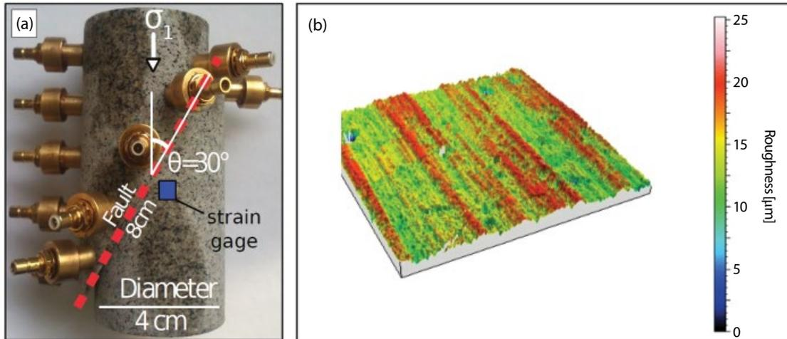
**Figure 12.1** Experimental setup. (a) The fault system is simulated using a saw cut Westerly granite sample. The fault is inclined at an angle  $\Theta = 30^\circ$  to  $\sigma_1$ . Blue square refers to the location of the strain gauges used to estimate the friction coefficient at the onset of instability and the dynamic stress change. (b) Measurement of the initial roughness of the fault surface. See *electronic version* for color representation.
