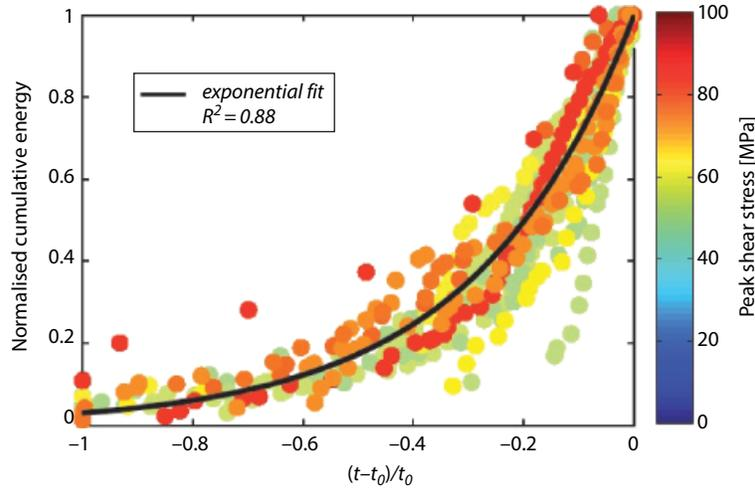
**Figure 12.8** Normalized cumulative acoustic energy released as a function of normalized time for 20 stick-slip cycles. Foreshock sequences collapse to an exponential law (black solid line) with  $\alpha \approx 3.5$ . See *electronic version* for color representation.
