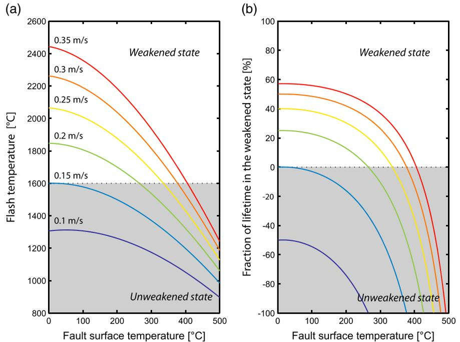
**Figure 4.** The influence of ambient fault surface temperature on flash-heating behavior. (a) Influence of fault surface temperature on the flash temperature of an asperity; estimates for quartzite for different indicated slip rates. (b) Influence of ambient fault surface temperature on the fraction of its lifetime an asperity spends in its weakened state; estimates for quartzite, for the same slip rates indicated in Figure 4a.
