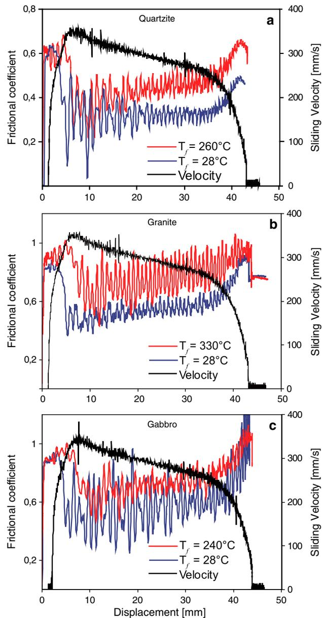
**Figure 1.** Effect of sliding velocity (black trace) on friction during experiments conducted at  $T_f \approx 25^\circ\text{C}$  (blue trace) and  $T_f \approx$  (indicated higher temperature) (red trace). Plots are for (a) quartzite, (b) granite, and (c) gabbro.
