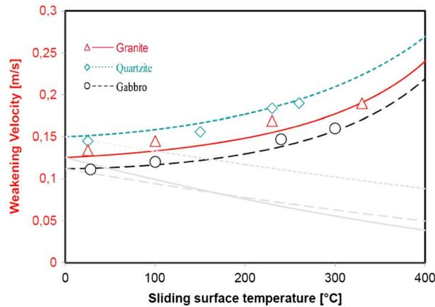
**Figure 3.** Influence of average fault surface temperature on the weakening velocity. Blue, black, and red lines and symbols represent, respectively, the theoretical estimations and experimental data for the weakening velocity for quartzite, gabbro, and granite. Gray dashed lines correspond to the theoretical predictions made without taking into account the influence of ambient fault temperature on the values of various physical parameters.
